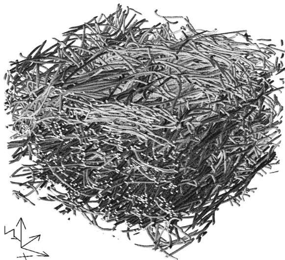
Figure 1. 3-D reconstructed DVI image of a typical carded hydroentangled nonwovens ( 800 \times 800 \times 600 voxels, with a resolution of 1.77 \mu\text{m}/\text{pixel} and an average fiber diameter of about 15 \mu\text{m} ).
